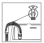
If it is placed over the edge of a basin or sink be sure the free end of the hose should not be underwater.
